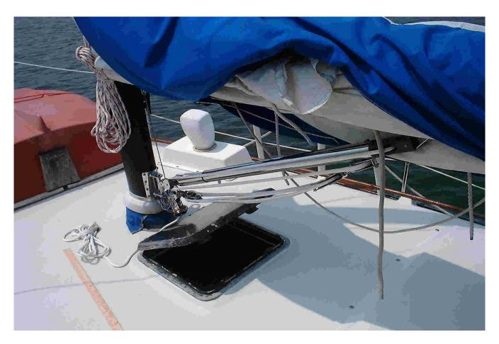
I then applied a thick bead of LifeSeal (a poly/silicone blend) all around the frame and, remembering to make it face backward, placed the frame in place. I then tightened the screws down minutes before Mike arrived to install the vang. I forgot the step in which you leave the screws partially tightened for 24 hours and then tighten the rest of the way after the sealant has cured. I hope I don't suffer as a result!
