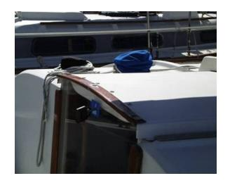
Mine was badly weathered and needed replacing. I did not like the original design since I could never get a good grip on it to close the hatch. Rather than replacing with a copy of the original, I designed a larger one that I could get a grip on and which would deflect any green water that made it over the sea hood (Figure 2).
