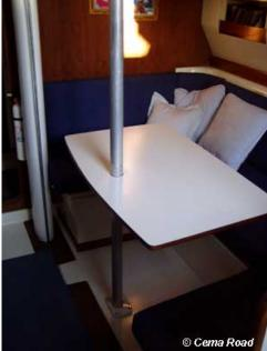
The design of the settee table on the 323 is not particularly robust. I've heard stories from other owners about how theirs can swing like a pendulum on a clock. Not only is this a messy situation. It could be hazardous to anyone below, especially at dinnertime when four people are sawing on their steaks at the same time.
