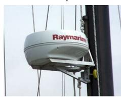
The Radar dome is on most boats is normally positioned either up the mast (right in the way of the crane when stepping), on a pole at the stern, or on the backstay. All of them have disadvantages and on the Great Lakes, the Radar is only needed a small fraction of the time. When we do get "socked in", it is a great asset.
