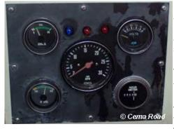
Installation was a snap. I drilled three holes just above the rev counter and slid two red, for the bilge pumps, and a blue, into place after putting some LifeSeal on the collar of each light. I then ran the wires along the inside of the engine room wall to the back of the bilge pump switches, connecting them to the same terminals used by the original light. That was it. I ran the blue light leads to the switch on the pressure water pump. I think the whole job took about 1 hour.
