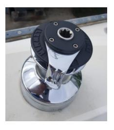
chrome platter and dropped off the drums. He glass beaded the drums (a form of sand blasting which is less aggressive) and to my surprise returned the gripping pattern to the middle of the drum. I scraped off the gross corrosion from the Aluminum parts with a small straight blade screw driver and then scotch-brighted all surfaces.
