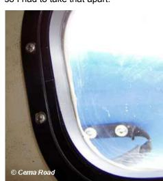
The two halves of the aluminum frame are held together with a total of four screws and two metal tabs that I then undid. With a little muscle, the metal pulled away
