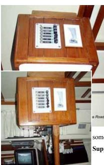
also the conduit for many of the cables that exit the cabinet. It appears to be a 2" square piece of teak (\$!) just shy of 2 feet in length. The center section of the pole was lathed round, which makes a good hand hold when moving around the cabin. There is a channel that is about 1/2" in diameter that runs down the center of the pole that handles some of the cables. The 12v power, ground and VHF antenna cable feed up through this opening.
