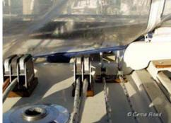
To port of the companionway, crew can control the traveler, main sheet, boom vang, jib and spinnaker halyards. Two single-speed winches make
