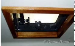
I screwed and glued two small pieces of scrap wood above the liner on the starboard and port side of the opening. To these I screwed the frame from inside the opening. It fit perfectly... almost. What remained was a gap between the top of the frame and deck above. A trip back to Ace Hardware found some thick and wide closed cell adhesive weather stripping that I stuck to the bottom of the decking. This closed the gap above the frame and completed the job.
