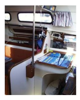
To align it I used a plumb bob from the upper connection to find where the hole should be drilled in the teak block. To hold the tube in place within the teak block I used two #10 stainless screws with barrel nuts to give it a professional finish. The block was secured to the bulk head with two ¼ inch bronze lag bolts. These are hidden by the removable seat back cushion. The bottom of the teak block was cut to match the other curved edges in the cabin.
