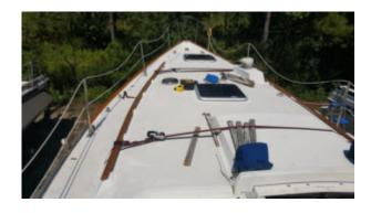
pedestal and drilled a smaller hole in the fiberglass and attached the screw. The only reason this worked is that there is an odd number of pedestals so the center is easy to find. I attached ratchet straps to the starboard rail aft and starboard stanchion forward. This allowed me to easily bend the handrail for the next pedestals fore and aft. I went fore and aft one by one, slowly bending and attaching the handrail. Once the port side was complete I moved everything to the starboard side.
